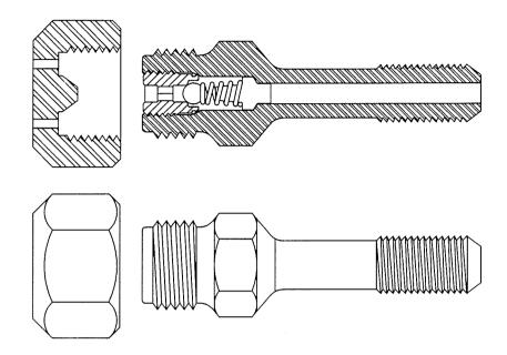
Long Stems Coupled With Parallel Threads are Available to Suit Any Requirement.
